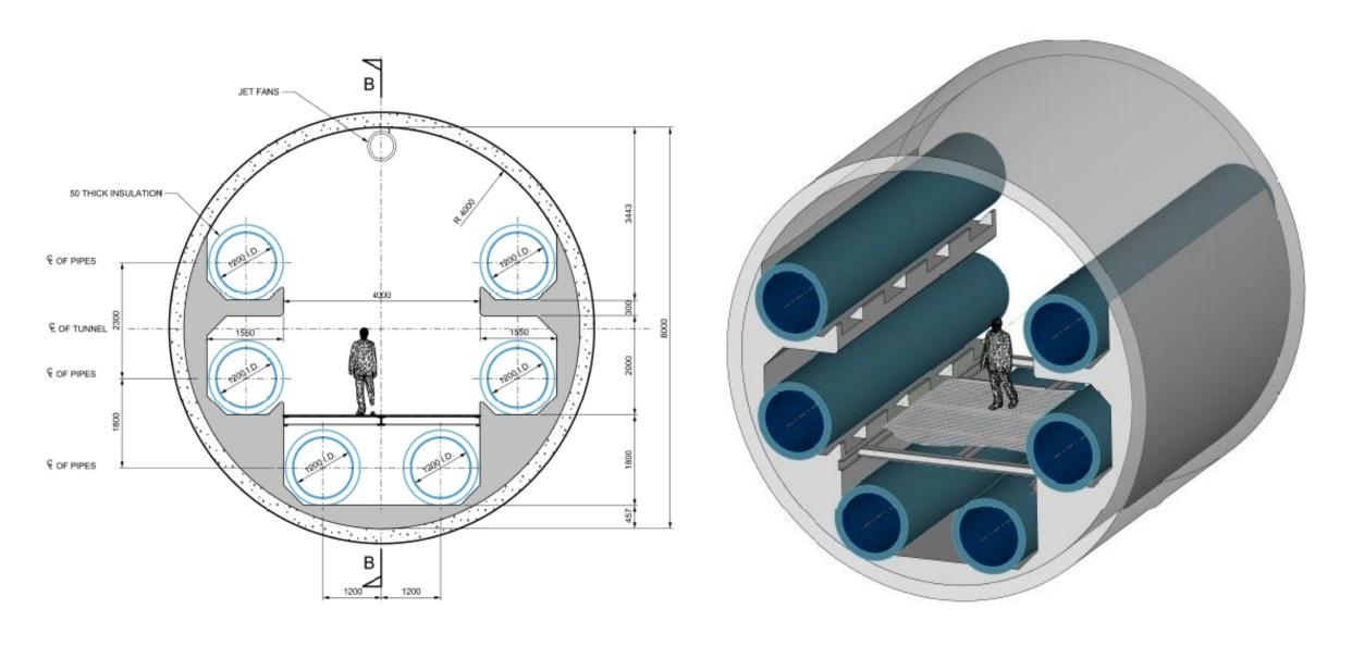
Cross section for 8m diameter pipe carrying 6 x DN1200 DH pipes
